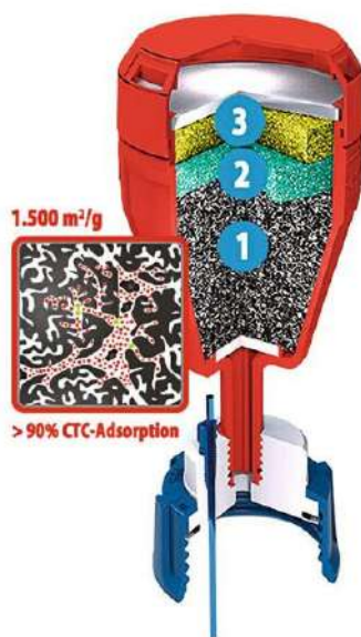
Fig. 2: The Safety Waste Caps contain three different types of activated carbon for additional safety: 1st layer adsorbs solvent vapours, 2nd layer binds alkalis, 3rd layer binds acids.
